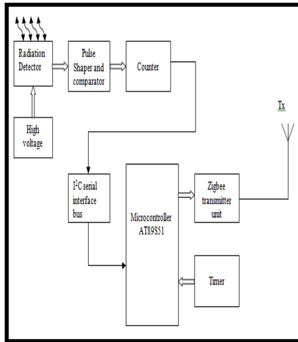
Fig no.1 Monitoring unit to detect radiation
