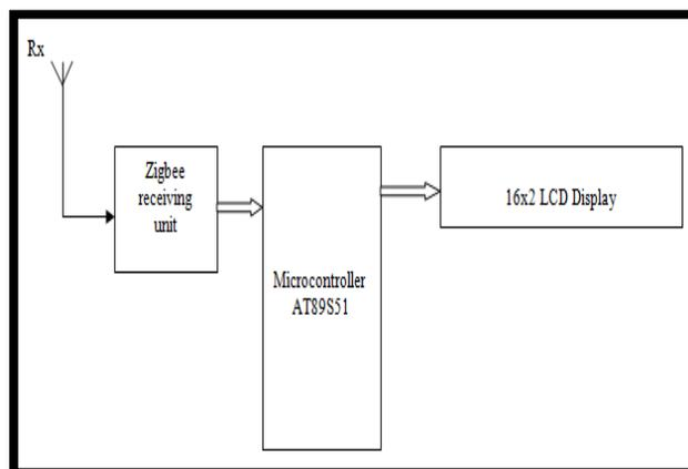
Fig no.2 Readout unit to display measured radiation
